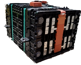
Figure 4: A battery module at Rejoule facility consisting of multiple cells
